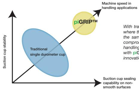
With traditional single durometer cups, where the lips and bellows are made of the same material, you either have to compromise on the grip or the machine handling speed. That is now history with piGRIP<sup>TM</sup>, the efficient automation innovation from Piab.
