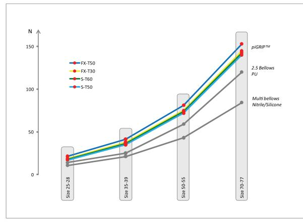
Proven function and lifting capacity within specified area of operation. See suction cup selection guide on www.piab.com for specified performance data.
