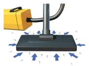
A vacuum cleaner does not suck. Air and dust are pressed into the vacuum cleaner by the surrounding higher atmospheric pressure.
