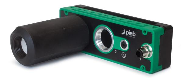
It is available with a three-stage COAX® cartridge MIDI. Choose an Si cartridge for extra vacuum flow, a Pi cartridge for high performance at low feed pressure or an Xi cartridge when high flow and deep vacuum is needed. This pump has a substantially lower air consumption compare to competition, it is compact with no moving parts. It can be configured with 1–6 cartridges. This pump can easily be upgraded with more capacity if needed. And it is also easy to disassemble for maintenance.
