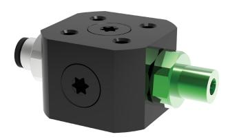
This is a fully decentralized vacuum unit based on patented COAX® technology. It provides the quickest response time and very high energy efficiency. The COAX® in piGRIP® is available with a variation of two stage COAX® MICRO cartridges. The COAX® in piGRIP® is compatible with any suction cup with G1/8" male fitting.
