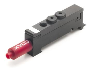
Compact/stackable vacuum pumps are air-driven multistage ejector families, based on COAX® technology, they are equipped with integrated controls and special functions, such as on/off valve, blow-off valve, vacuum switch, energy saving function etc. They are configurable platforms, making it easy to specify the exact control functions needed for the system.
