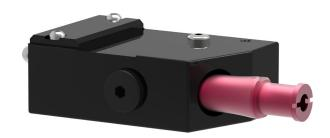
This is a product design where different suction cups can be integrated with vacuum cartridges based on the patented COAX® technology. The "vacuum gripper" makes selection, sizing and installation of a vacuum system easier. With a VGS™ you will enjoy the benefits of a more cost-efficient and reliable decentralized vacuum system. The VGS™ is compatible with any suction cup with G3/8" male fitting. It has a low weight at 204–340 g.
