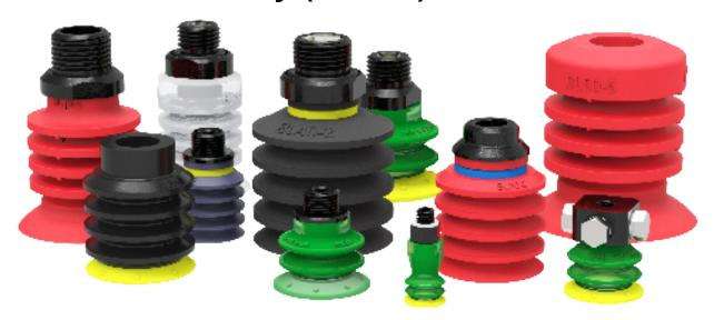
This family is designed for height differences, slightly curved planes and uneven surfaces. Applications such as bag handling, cardboard, high temperature or if the need is specifically to touch a food item as they are also available in material that complies with the FDA (FDA 21 CFR 177.2600) and meets EU's regulation EU 1935/2004.
