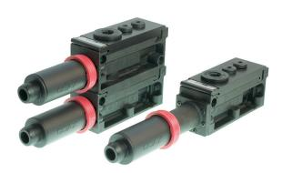
Compact/stackable vacuum pumps are air-driven multistage ejector families. based on COAX® technology. they are equipped with integrated controls and special functions. such as on/off valve. blow-off valve. vacuum switch. energy saving function etc. They are configurable platforms. making it easy to specify the exact control functions needed for the system.
