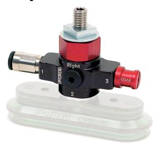
Piab VGS<sup>™</sup> – A product design where different suction cups are integrated with vacuum cartridges based on the patented COAX® technology. The "vacuum gripper" makes selection, sizing and installation of a vacuum system easier. With a VGS<sup>™</sup> you will enjoy the benefits of a more cost-efficient and reliable decentralized vacuum system. It has a low weight at 25–39 g.
