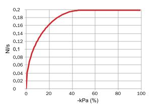
At 47 -kPa the air reaches sonic velocity, and consequently the flow is constant.
